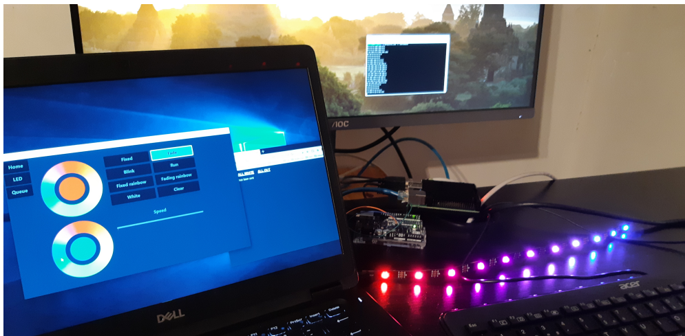
JavaFX on PC, terminal on Pi with Mosquitto and Arduino with LED strip
