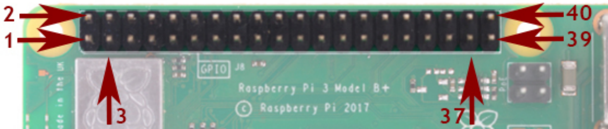
Pi pin header with the indication of pin 1, 2, 3, 37, 39 and 40
