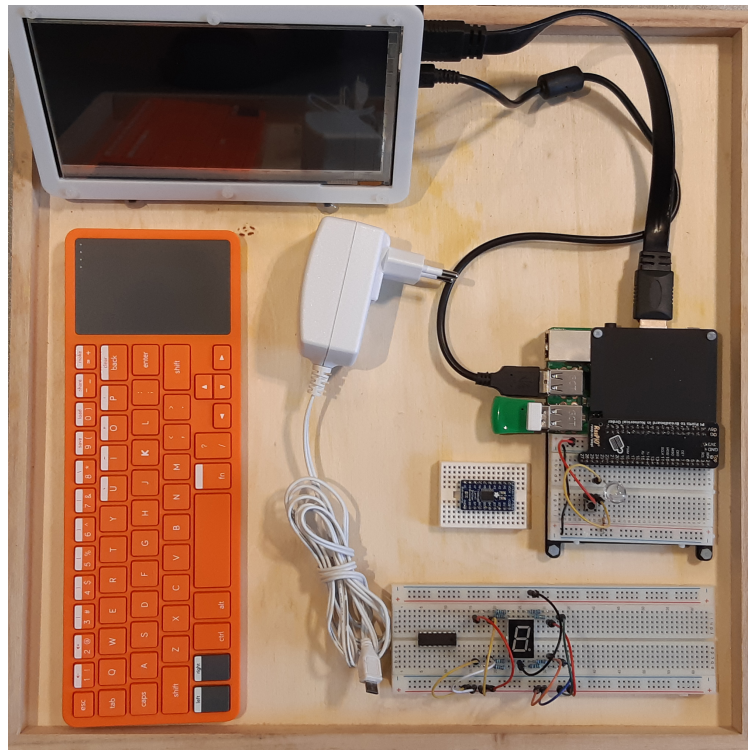
Pi 3 test setup with multiple breadboards
